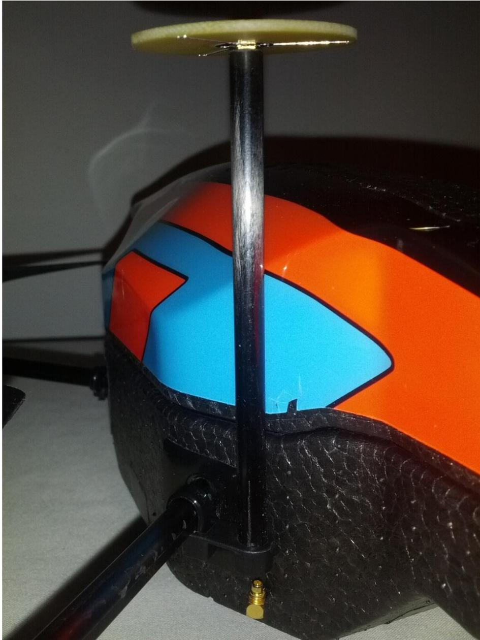
**Bottom Mount – In Flight:** (Velcro used to secure to Bottom Cover)
